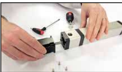
Insert motor shaft into coupling
