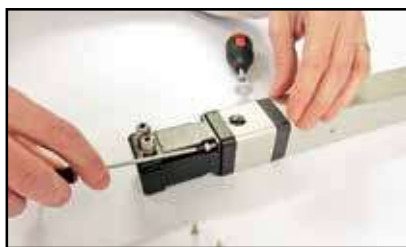
Tighten motor mounting screws
