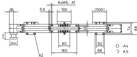
RediMount Flange SpecificationsParameterMinMaxFlange length (Lrm)[mm]83145Flange square (Srm)[mm]90200Flange weight \*[kg]5,64
